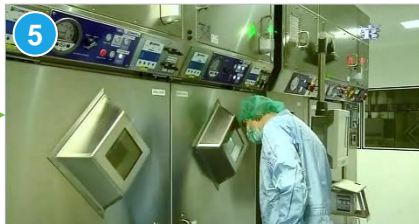
5 Radioactive liquid is dispensed by automatic dispenser
