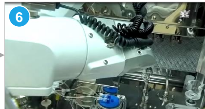
6 The machine automatically issues tungsten vials
