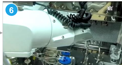
6 The machine automatically issues tungsten vials
