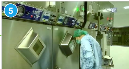
5 Radioactive liquid is dispensed by automatic dispenser
