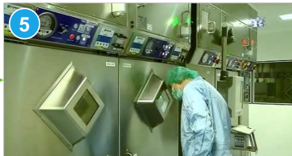
5 Radioactive liquid is dispensed by automatic dispenser
